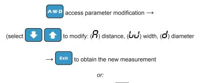
pull out the gauge to repeat the measurement  $\rightarrow$  **Exit** to obtain the new measurement.
