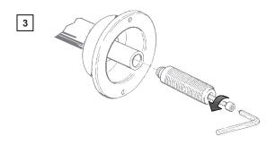
The wheel balancer is supplied complete with cone type adapter for fastening wheels with central bore. The threaded terminal is fitted according to the drawing; it can be removed to fit optional adapters.
